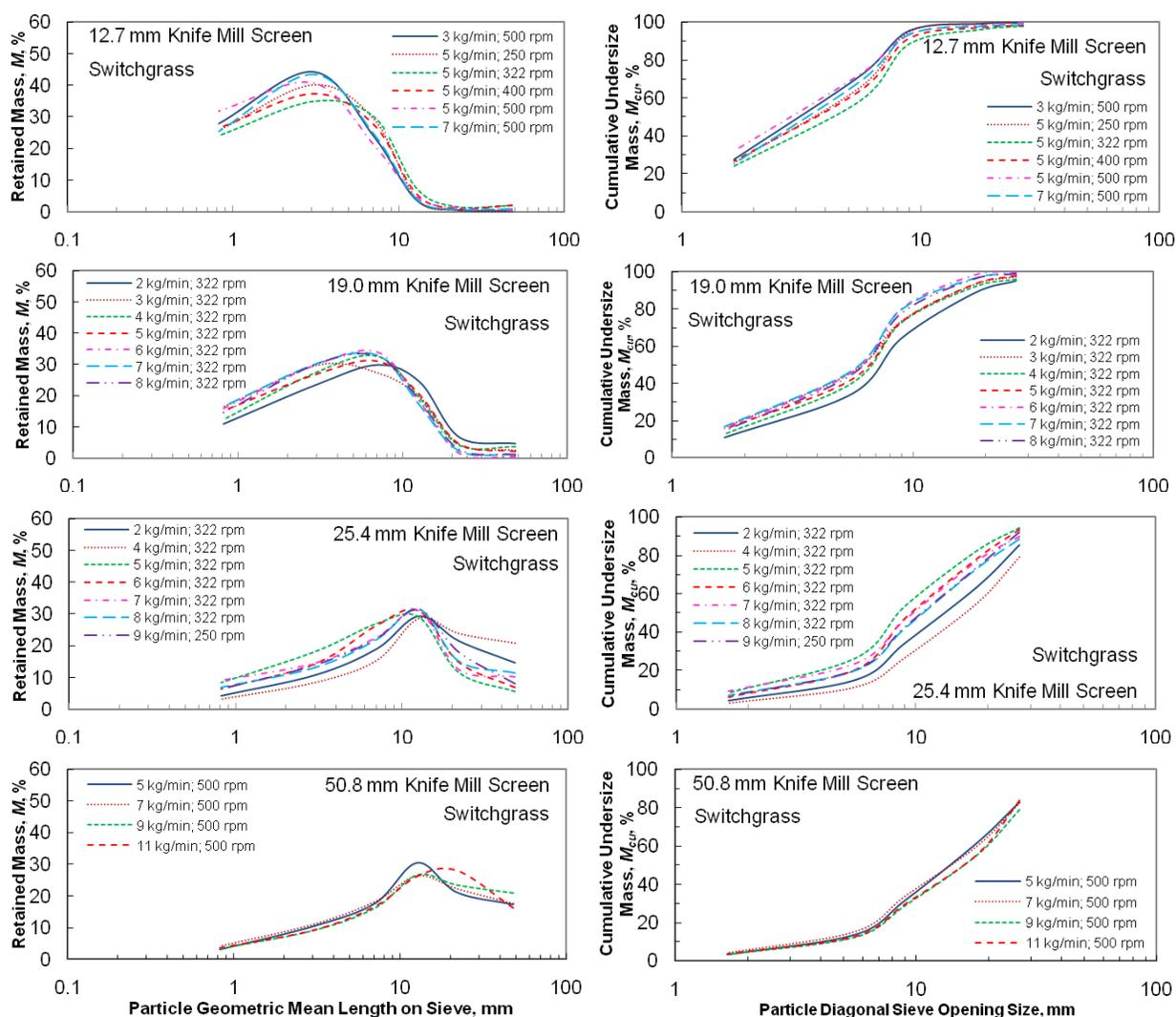
Figure 9. Log-normal distribution and cumulative percent undersize of chopped switchgrass.
